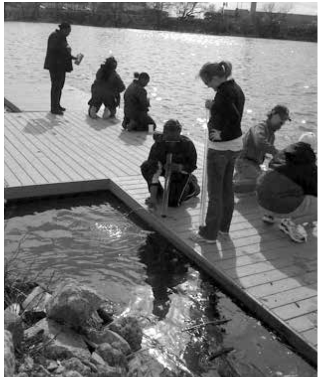
Figure 14. Roosevelt students and faculty performed several tests of Bubbly Creek's water quality. The most significant finding was a level of fecal coliforms well beyond the safe limit for boating or swimming. Photograph by Carl Zimring.
